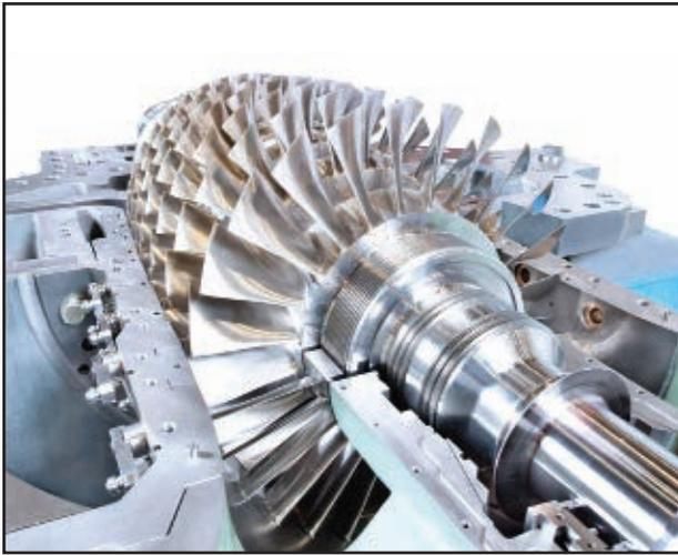
The seven-stage MAX1 axial compressor with top casing removed, showing blade configuration.
