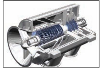
AR compressor for air separation production of 5512 tons/d (5000 tonnes/d) oxygen at 305 psi (21 bar).
