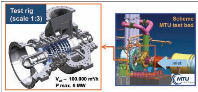
Schematic of test rig alongside the MTU test bed showing direction of air flow.
