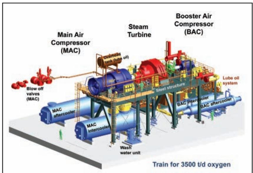
Computer rendering of an air separation unit (ASU) compressor train with a steam turbine driving both a booster compressor and a main air compressor. This train is for application on very large air separation units with an oxygen-producing capacity of 3858 tons/d (3500 tonnes/d).
